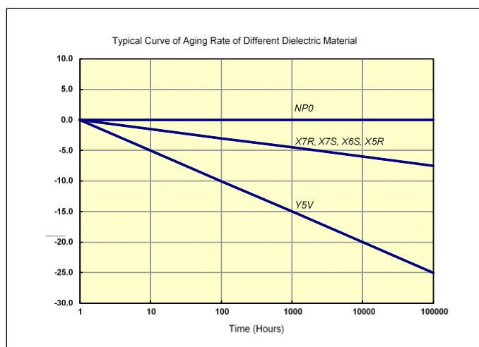
$$C_{t2} = C_{t1} \times (1 - k \times \log_{10}(t_2/t_1))$$
