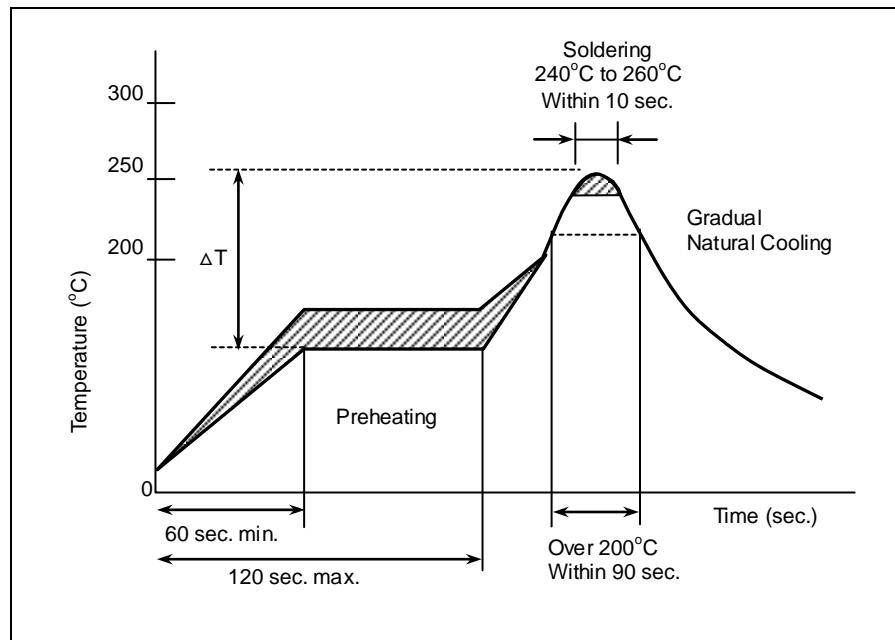
The difference between solder and chip surface should be controlled as following table. The rate of preheat should not exceed  $4^{\circ}\text{C/sec}$  and a target of  $2^{\circ}\text{C/sec}$  is preferred.
